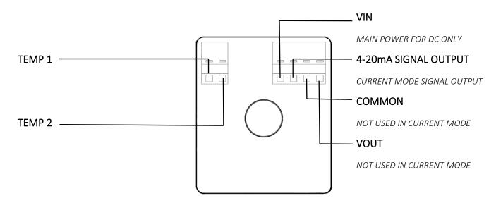
Temp Element: Interchangeable NTC thermistor, 2-wire
